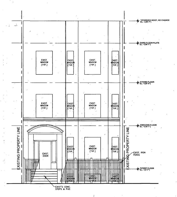
FRONT ELEVATION W/ EXISTING CONCRETE STEPS/ FENCE
