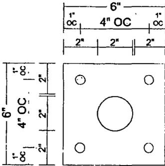
6" x 6" x .500 steel plate with welded ø2" pipe,
