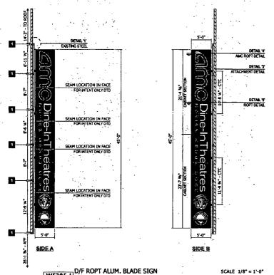
WF205-1 ONE (1) REQUIRED - MANUFACTURE AND INSTALL
