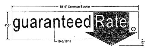
Fabricated 3" deep aluminum common back panel mounted to brick building facade with necessary anchors, secured through pan returns
