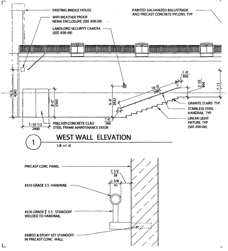
HANDRAIL DETAIL @ PRECAST CONCRETE WALL TYP.
