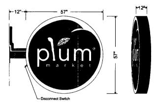
12" deep fabricated aluminum blade sign, 090 Aluminum return with .1875 #7328 translucent white acrylic faces, with respective color vinyl graphics applied 1" std white timicap. Returns painted PMS 222C Steel structure included for mounting to 5" x 5" x 3/16" tube
