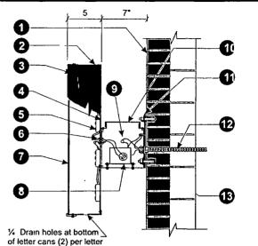
Section @ LED Channel Letter Raceway mount installation
