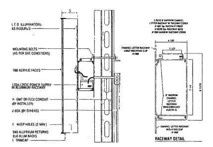
DETAIL FOR TYPICAL RACEWAY MOUNTED CHANNEL LETTER WITH ILLUMINATED PLEX FACE
