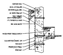
SECTION DETAIL @ CHANNEL LETTERS SCALE 1 A 1 0
