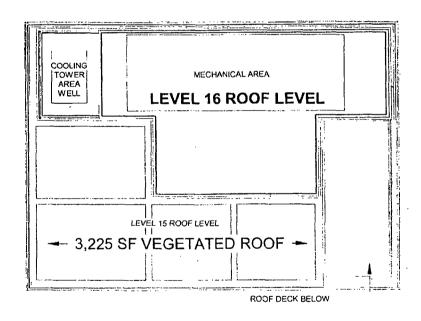
Total Non-Mechanical Roof Area = 7,850 SF Total Green Roof Area = 3,935 SF Green Roof Area > 50% of Total Non-Mechanical Roof Area
