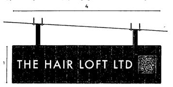
Sign- 4 sq ft - 65 lbs Total Wattage 18 watts LED illuminated One (1) 24 volt power supply Toggle switch side of sign
