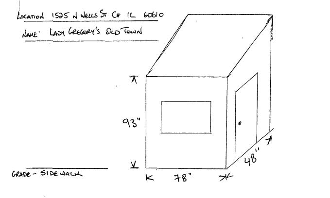
HEIGHT OF STRUCTURE - 93" DEPTH OF STRUCTURE - 48" CENGTH OF STRUCTURE - 78"
