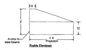
Shed style awning with closed ends fabricated with mill finish mig-welded aluminum frames with added 1x2 construction
