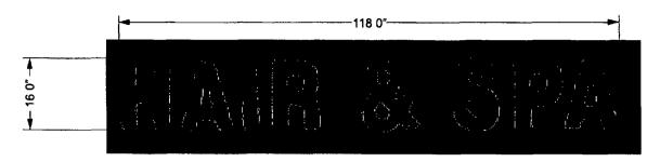
Front-Lit, Plex-Face Channel Letters w/ Backplate and LED, Wireway Mounted • Front View SCALE 0/0 = 1'0' For Production / For Presentation
