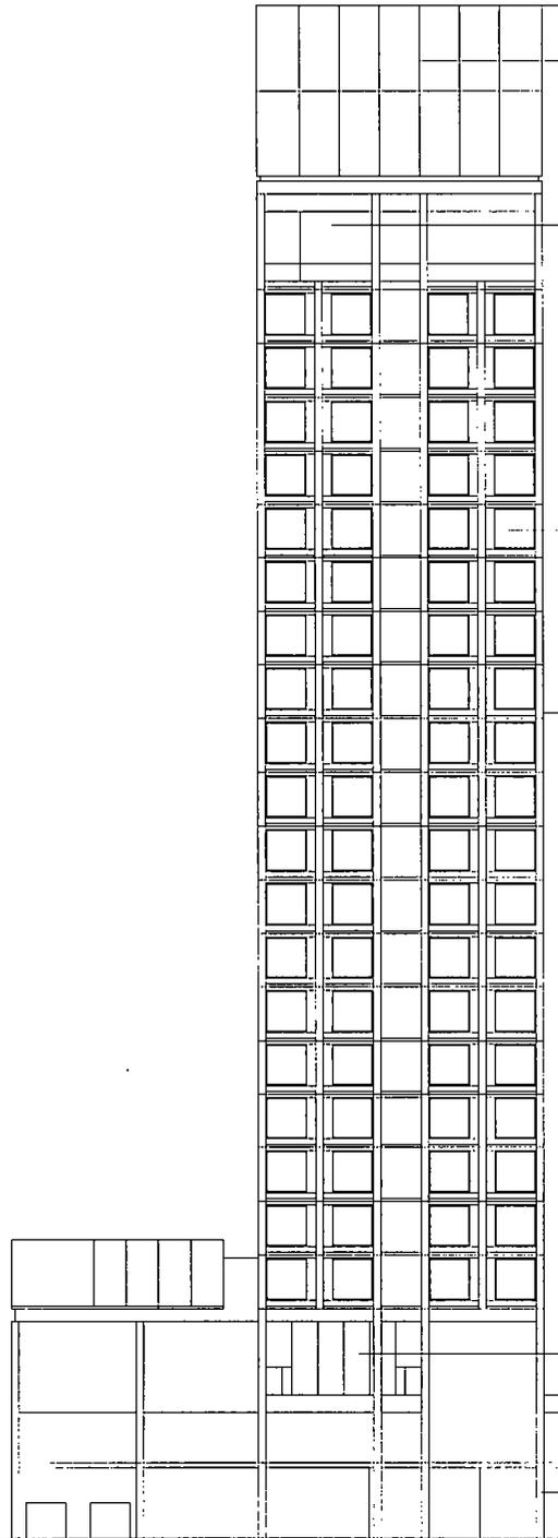
CLEAR LOW-IRON, LOW-E COATED IGU WITH LAMINATED INNER LITE AND CUSTOM PATTERN ACID-ETCH COATING
