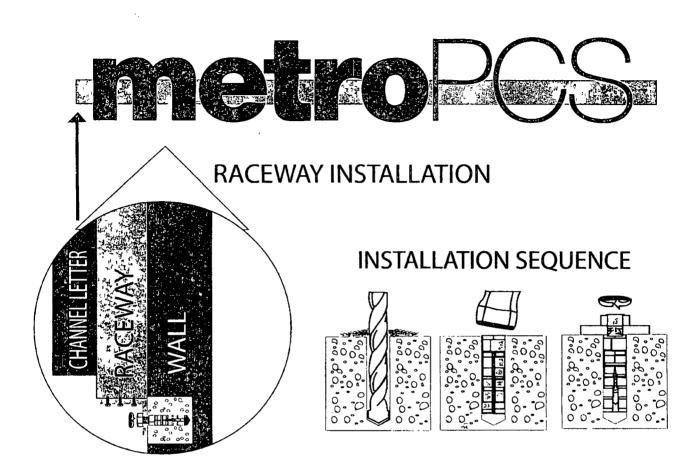
MATERIAL FOR INSTALLATION HEX-BOLT 5/16" X 3" LAG SCREWS 3/8" X 3" SELF-DRILLING SCREWS #10 3/4" SHORT LAG SHIELDS 3/8" X 1-3/4" L BRACKET 1"X4" LONG
