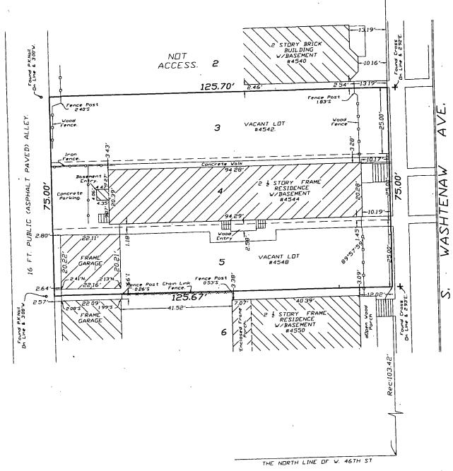
MONUMENTATION OR WITNESS POINTS WERE NOT SET AT THE CLIENTS REQUEST. UNLESS OTHERWISE NOTED HEREON THE BEARING BASIS, ELEVATION DATUM AND COORDINATE DATUM IF USED IS ASSUMED.
