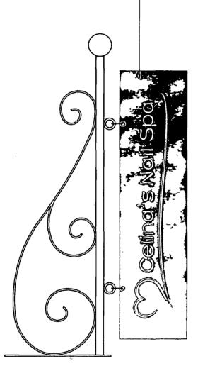
aluminum panel painted custom 3/8' (dia) lag bolts 3" embed 9" (h) X 36" (w) X 1/8" (thick) turquoise (paint match TBD) matte black steel decorative sign bracket which attaches Matte gold vinyl logo on both sides installed with to masonry facade with
