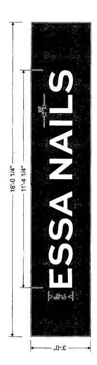
Back-Lit Channel Letters On Wireway • Pin Mounted • Front View SCALE 1/2 = 1 For Production / For Presentation
