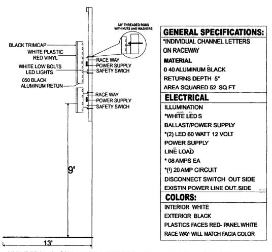
\*INDIVIDUAL CHANNEL LETTERS 15IN AND 14IN BOTTOM PANEL \*ATACHED TO THE WALL WITH THREADED ROT NUTS & WASHERS \*EXISTING POWER LINE OUT SIDE
