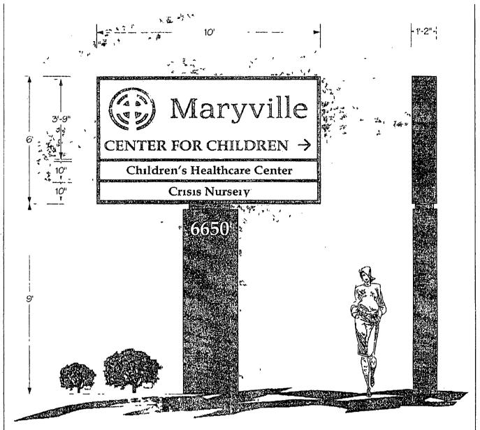
A COMPLETE INTERNALLY ILLUMINATED PYLON SIGN ALL LED INTERNALL LIGHTING COMPONENTS ALL NEW CONCRETE FOUNDATIONS' STEEL SUPPORTS AND POLE SKIRT INDIVIDUAL CHANGEABLE DIRECTIONAL PANEL AREAS
