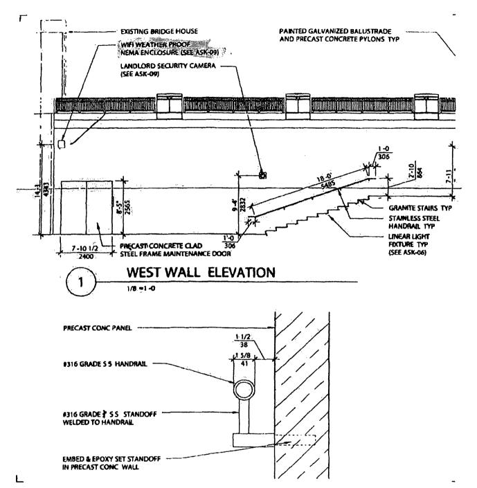
HANDRAIL DETAIL @ PRECAST CONCRETE WALL TYP.
