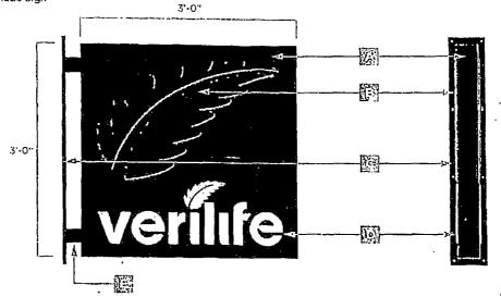
36" (sq.) X 3" (deep) double-sided, fabricated, internally LED-lituminated sign cabinet. All exposed surfaces painted standard black
