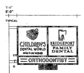
1 1/2" X1 1/2 "X 3/16" GALV. ANGLE IRON FRAME / WELDED 1 1/2" X 3/8" GALV. BOLTS 20 GAUGE GALV. DRUM 2" X 2" GALV. 20 GA. TRIM 1/2" DRAIN HOLES 5/18 LEXAN SIGN PROJECTING
